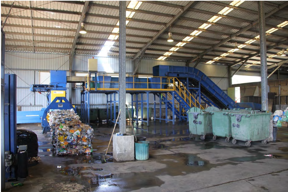
Figure 3.3: Multi-Purpose Baler and Mini Sort Line used for aluminium, steel, plastic and residual wastes at the WMC
